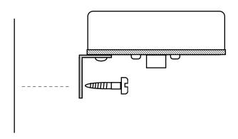
**Important Note**: Always mount with the connectors facing downward to ensure maximum protection from water incursion.
